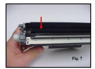
8. Clean the doctor blade with compressed air. Using a cotton swab with 99% IPA, clean the leading edge of the doctor blade (Fig. 8).
